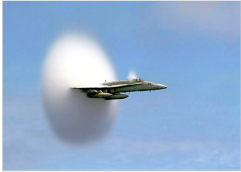
U.S. Navy F/A-18 approaching the sound barrier. The white cloud forms as a result of the supersonic expansion fans dropping the air temperature below the dew point. [1][2]
