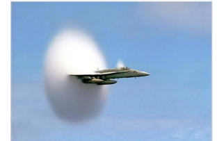
U.S. Navy F/A-18 approaching the sound barrier. The white cloud forms as a result of the supersonic expansion fans dropping the air temperature below the dew point. [1][2]
