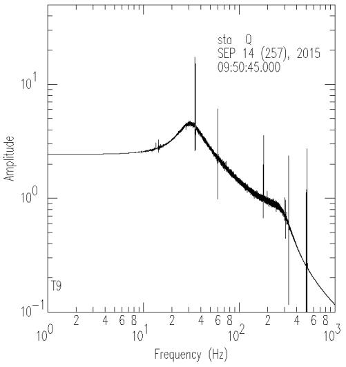
Based on the above FFT plot, and the spectrogram plot next page, we can see that there are peak noises in the following frequency ranges (20-80 Hz, including 35 Hz, 60 Hz), 180 Hz, and 330 Hz. In addition, there is a minor vertical stripes (the targeted signal) between 70-300 Hz.
