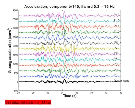
2). According to the Table 2 of the Fletcher et al. (BSSA, 2006) paper, the best-fitting apparent velocity  $C_{app}$  and back-azimuth  $\theta$  for the following time window [34.1 – 34.6] s (the time window corresponds to data at the center station P06) is:  $C_{app} = 2.75$  km/s,  $\theta =$
