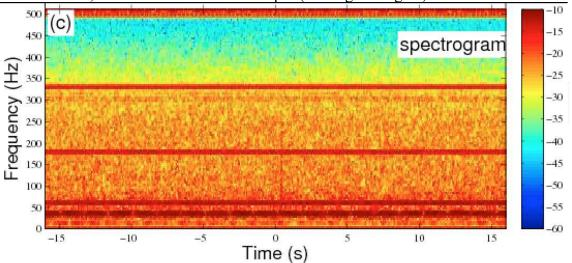
Hence, we apply a band-pass-filter of 80-300 Hz, and a notch filter (band-rejected filter) between 178-182 Hz and 329 to 333 Hz. See gen\_spectrogram\_Livingston.m for more details.
