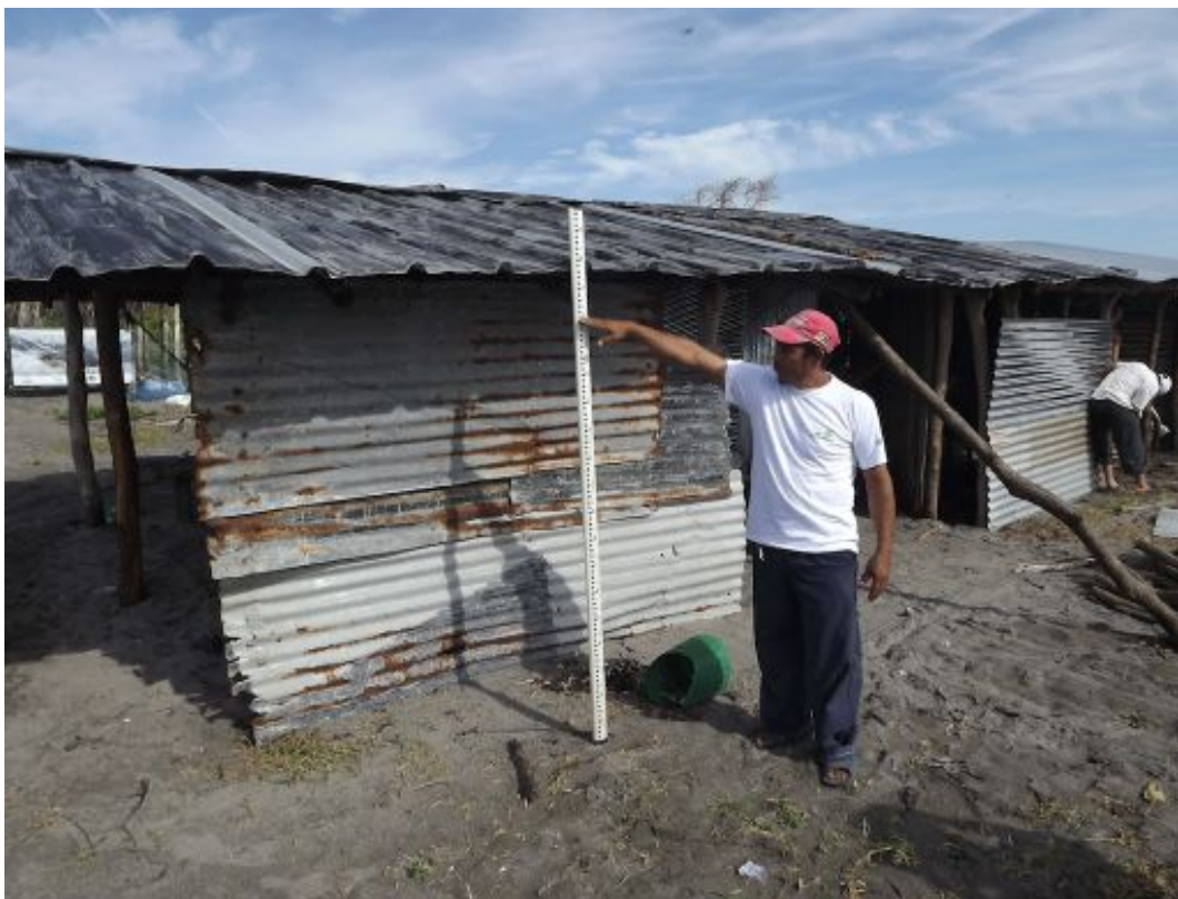
Figure 3.18 Resident at Mangalrón indicates the flow depth at the site. The walls of the shed had been ripped off by the tsunami and replaced since the event.
